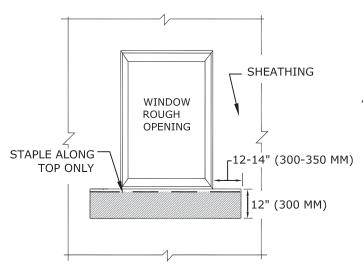
CUT STUCCOWRAP APPROXIMATE SIZE SHOWN AND STAPLE INTO PLACE AT BOTTOM OF THE ROUGH OPENING.
